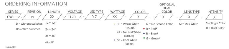
CWL-D-48-120-0-7-40-50-M-S - CWL D Type, 48", 120VAC, 40W, Cool White, Milk White Lens, Single Intensity Lens
